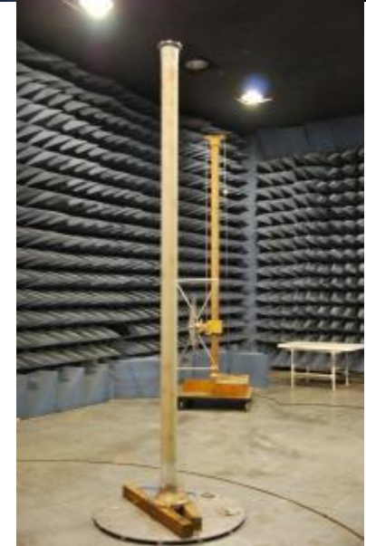
AS-1096/URC Antenna - Anechoic Chamber Testing for E / H Plane Patterns, Return Loss, VSWR
