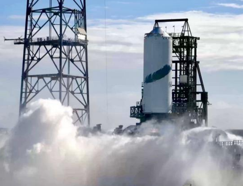
Hot-fire Testing of New Glenn Second Stage
