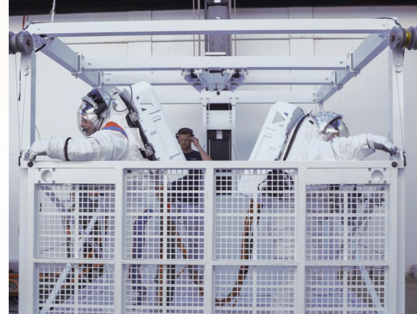
Pressurized Suit-Elevator Operations Testing
